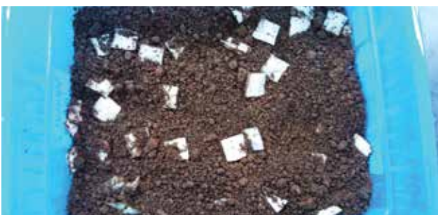
Figure 2: The biomass plate before and after 90 days of incubation
