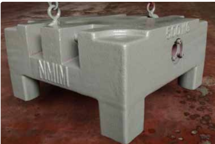
CAST IRON STANDARD WEIGHT FOR NMIM
