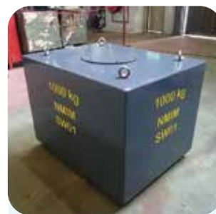
1,000 kg standard weight fabricated by FTS for the National Metrology Institute of Malaysia
