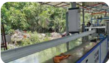
Continuous production of 160 mm diameter composite pole for solar streetlight
