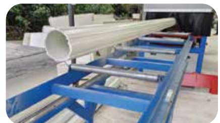
Continuous production of 160 mm diameter composite pole for solar streetlight
