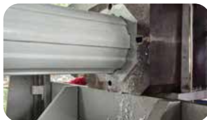
Continuous production of 160 mm diameter composite pole for solar streetlight
