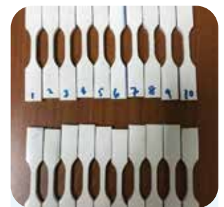
Test specimen machined by FTS for Plastics and Composites Material Section, SIRIM QAS International Sdn Bhd
