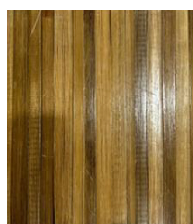
Untreated bamboo laminated composite
