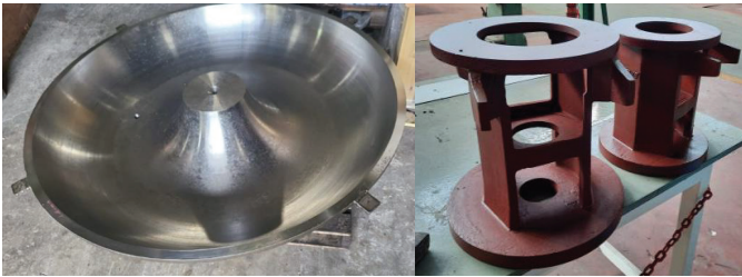
Cast bowl and mixer bracket for food processing machinery
